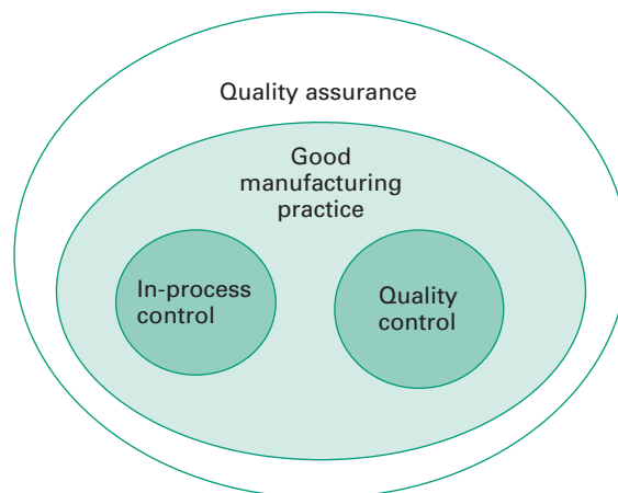
Figure 23.1 The inter-relationship between quality assurance, good manufacturing practice, quality control and in-process control.
